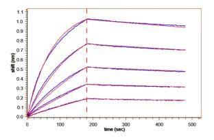
Loaded Anti-A2AR Antibody on Protein A-Biosensor, can bind Human A2AR Nanodisc, His Tag with an affinity constant of 4.44 nM as determined in BLI assay (Gator).
