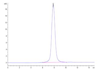
The purity of SARS-CoV-2 Spike S1 (Omicron BA.2.12.1) is greater than 95% as determined by SEC-HPLC.
