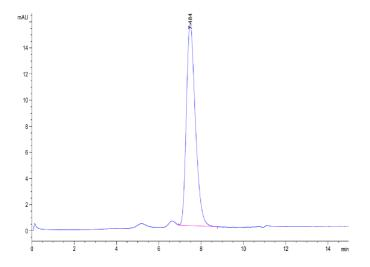
The purity of Human BCMA is greater than 95% as determined by SEC-HPLC.
