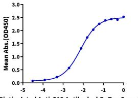
Immobilized Human CA9, hFc Tag at  $1\mu$ g/ml (100 $\mu$ l/well) on the plate. Dose response curve for Biotinylated Anti-CA9 Antibody, hFc Tag with the EC50 of 7.4ng/ml determined by ELISA (QC Test).
