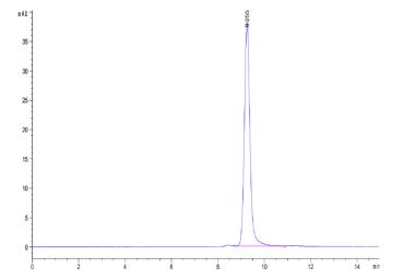
The purity of Mouse CCL24 is greater than 95% as determined by SEC-HPLC.
