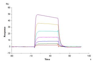
Cynomolgus IL-2 R beta, His Tag captured on CM5 Chip via anti-his antibody can bind Human IL-2, No Tag with an affinity constant of 0.17  $\mu$ M as determined in SPR assay (Biacore T200).
