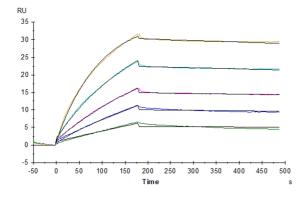
Biotinylated Human CD20 VLP, captured on CM5 Chip via streptavidin can bind Rituximab, hFc Tag with an affinity constant of 0.68 nM as determined in SPR assay (Biacore T200) (QC Test).
