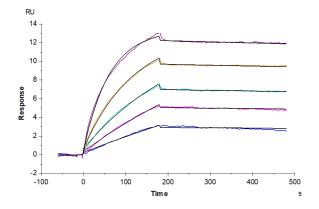
Biotinylated Human CD20 VLP captured on CM5 Chip via streptavidin can bind Ofatumumab, hFc Tag with an affinity constant of 0.61 nM as determined in SPR assay (Biacore T200).
