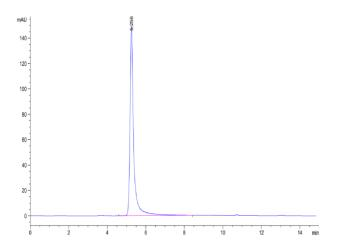
The purity of Biotinylated Human CD20 VLP is greater than 95% as determined by SEC-HPLC.
