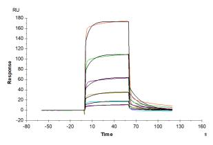
Human B7-1, hFc Tag captured on CM5 Chip via Protein A can bind Mouse CD28, His Tag with an affinity constant of  $5.12 \mu$ M as determined in SPR assay (Biacore T200).
