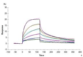
Biotinylated Claudin 18.2 Nanodisc, His Tag captured on CM5 Chip via Streptavidin can bind Anti-Claudin18.2 Antibody with an affinity constant of 12.50 nM as determined in SPR assay (Biacore T200).
