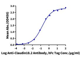
Immobilized Biotinylated Human Claudin 18.2 Nanodisc, His Tag at  $5\mu$ g/ml ( $100\mu$ I/well) on the streptavidin precoated plate ( $5\mu$ g/ml). Dose response curve for Anti-Claudin18.2 Antibody, hFc Tag with the EC50 of 0.15 $\mu$ g/ml determined by ELISA.
