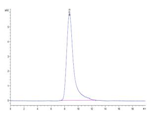
The purity of Human DLL4 is greater than 95% as determined by SEC-HPLC.
