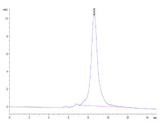
The purity of Mouse DLL3 is greater than 95% as determined by SEC-HPLC.
