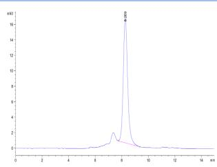
The purity of Human DSG3 is greater than 95% as determined by SEC-HPLC.
