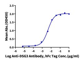
Immobilized Human DSG3, His Tag at 0.5µg/ml (100µl/Well) on the plate. Dose response curve for Anti-DSG3 Antibody, hFc Tag with the EC50 4.5ng/ml determined by ELISA.
