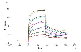
Mouse EGFR, His Tag captured on CM5 Chip via anti-his antibody can bind Mouse EGF, hFc Tag with an affinity constant of 3.98 nM as determined in SPR assay (Biacore T200).
