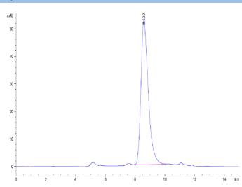
The purity of Human FAM3D is greater than 95% as determined by SEC-HPLC.
