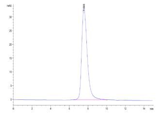
The purity of Biotinylated Human Fc gamma RIIIB (NA2) is greater than 95% as determined by SEC-HPLC.
