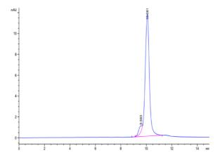
The purity of Cynomolgus FGF21 is greater than 95% as determined by SEC-HPLC.
