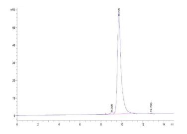
The purity of Cynomolgus FGL2 is greater than 95% as determined by SEC-HPLC.
