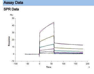
OKT3 captured on CM5 Chip via Protein A can bind Biotinylated Mouse Fc gamma RIII, His Tag with an affinity constant of 0.164  $\mu$ M as determined in SPR assay (Biacore T200).
