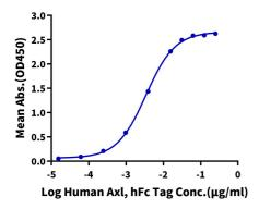
Immobilized Human GAS6, His Tag at 5  $\mu$ g/ml (100  $\mu$ l/well) on the plate. Dose response curve for Human Axl, hFc Tag with the EC50 of 3.4 ng/ml determined by ELISA (QC Test).
