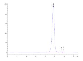
The purity of Human GCGR is greater than 95% as determined by SEC-HPLC.
