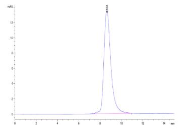
The purity of Mouse GEP is greater than 95% as determined by SEC-HPLC.  $\label{eq:continuous}$
