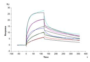
Human GPRC5D Nanodisc, His Tag captured on CM5 Chip via anti-his antibody can bind Anti-GPRC5D Antibody with an affinity constant of 1.47 nM as determined in SPR assay (Biacore T200).
