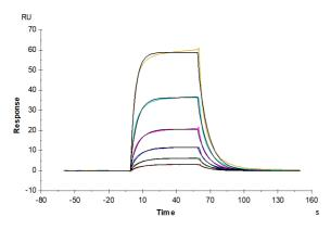
Human IL-3, hFc Tag captured on CM5 Chip via Protein A can bind Cynomolgus IL-3 R alpha, His Tag with an affinity constant of 0.46  $\mu$ M as determined in SPR assay (Biacore T200) (QC Test).
