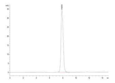
The purity of Rat IL-22R alpha 1 is greater than 95% as determined by SEC-HPLC.
