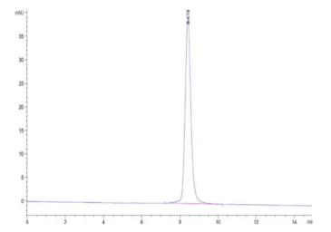
The purity of Mouse KLKB1 is greater than 95% as determined by SEC-HPLC.
