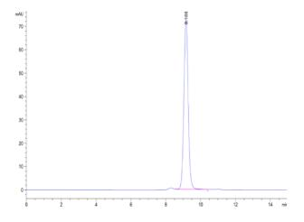
The purity of Human Peptide Ready HLA-A\*11:01&B2M Monomer is greater than 95% as determined by SEC-HPLC.
