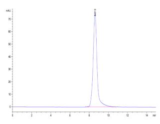
The purity of Biotinylated Human HLA-A\*02:01&B2M&HPV16 E7 (YMLDLQPET) Monomer is greater than 95% as determined by SEC-HPLC.
