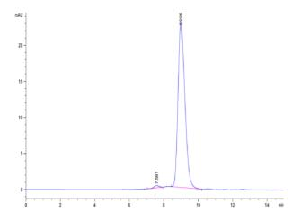
The purity of Cynomolgus PD-1 is greater than 95% as determined by SEC-HPLC.
