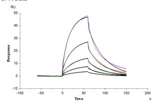
Mouse PD-L1, His Tag captured on CM5 Chip via anti-his antibody can bind Biotinylated Mouse PD-1, hFc Tag with an affinity constant of 3.35  $\mu$ M as determined in SPR assay (Biacore T200).
