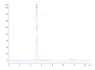
The purity of Human STEAP1 VLP is greater than 95% as determined by SEC-HPLC.
