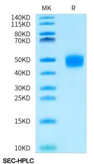
Cynomolgus Coagulation factor III on Bis-Tris PAGE under reduced condition. The purity is greater than 95%.
