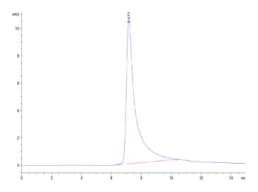
The purity of Human THSD7A is greater than 95% as determined by SEC-HPLC.
