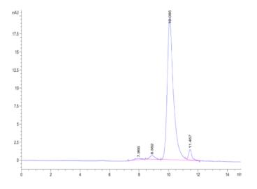
The purity of Biotinylated Cynomolgus TSLP is greater than 90% as determined by SEC-HPLC.
