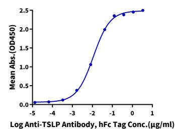
Immobilized Biotinylated Cynomolgus TSLP, His Tag at 0.5µg/ml (100µl/well) on the streptavidin precoated plate (5µg/ml). Dose response curve for Anti-TSLP Antibody, hFc Tag with the EC50 of 11.2ng/ml determined by ELISA (QC Test).
