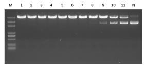
Results of a 30-minute digest reaction at 37°C with 1 $\mu$ g plasmid and 1 $\mu$ L Bsal (2-fold serial dilution in reaction buffer from lane 1 to lane 11, with lane 1 from 1  $\mu$ L 20U of Bsal, lane 2 from 1  $\mu$ L 10 U of Bsal, and so on) in a total reaction volume of 20 $\mu$ L. N is non-digested plasmid.
